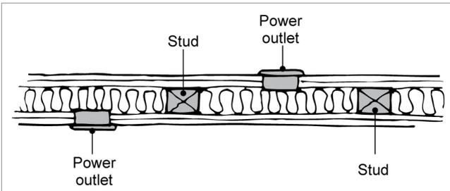
Offset power outlets to minimise noise leakage.
