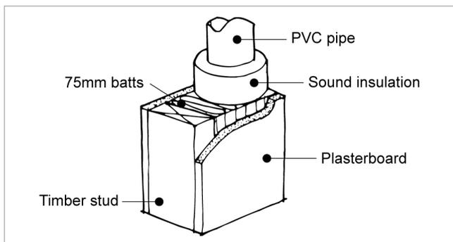
Sound-insulated plumbing in a stud wall.
