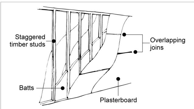
Offset plasterboard joints when layering the boards.
