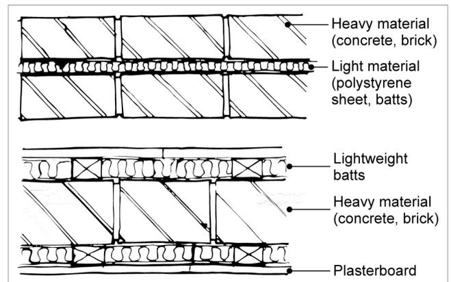
Composite constructions for reducing noise transmission.
