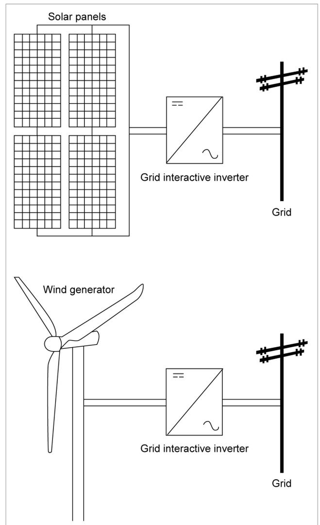
Both solar and wind generation systems can be connected to the grid.
