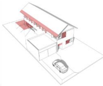
Concept sketches of key principles – design shaped to maximise northern exposure and preserve pleasant outdoor spaces, and various features used to shade windows from the summer sun.
